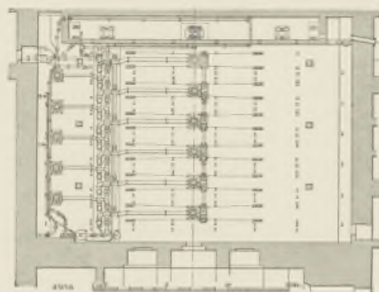
COURT THEATRE, BERLIN: STAGE. FIG. 104, 106. PLANS OF 'GRIDIRON' AND 'CABLES.'
