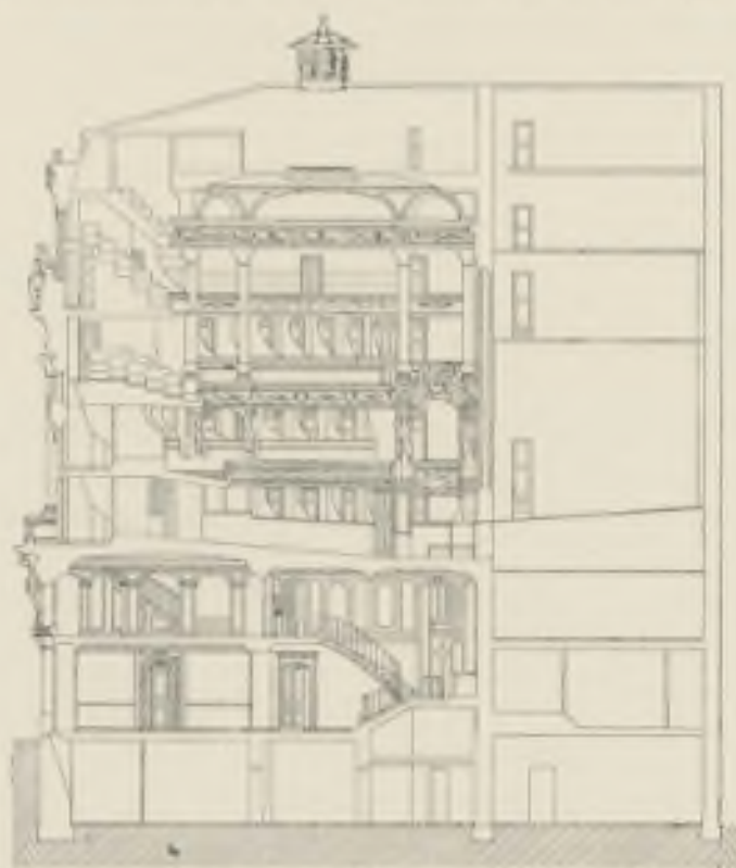
'RENAISSANCE' THEATRE, PARIS. FIG. 153. LONGITUDINAL SECTION.
