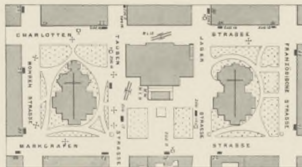
COURT THEATRE, BERLIN. FIG. 2. PLAN OF FIRE BRIGADE ARRANGEMENTS IN EVENT OF AN OUTBREAK.
