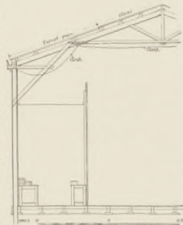
TEMPORARY THEATRE, PARIS (KNOWN AS "CHARITY BAZAR"). Destroyed MAY 4, 1897. FIG. 18. SECTION SHOWING ROOF, VELUM AND STALLS.
