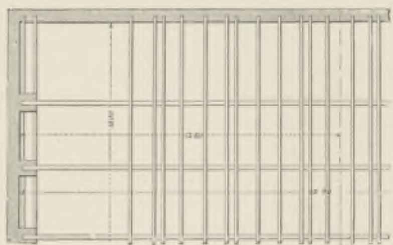
MUNICIPAL THEATRE, ROTTERDAM: STAGE. FIGS. 38, 39. PLAN OF 'FLY GALLERY' AND 'GRIDIRON.'
