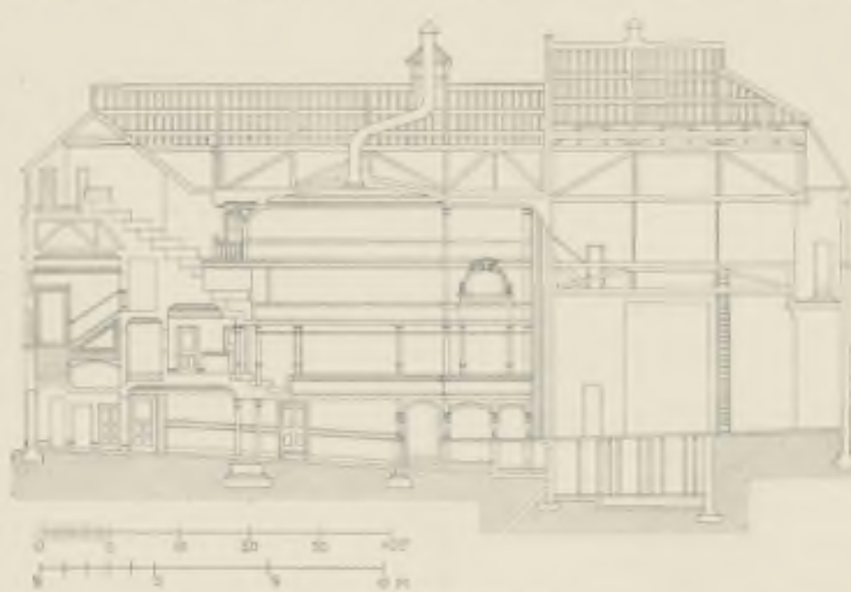
THEATRE, CHELTENHAM. FIG. 130. LONGITUDINAL SECTION.
