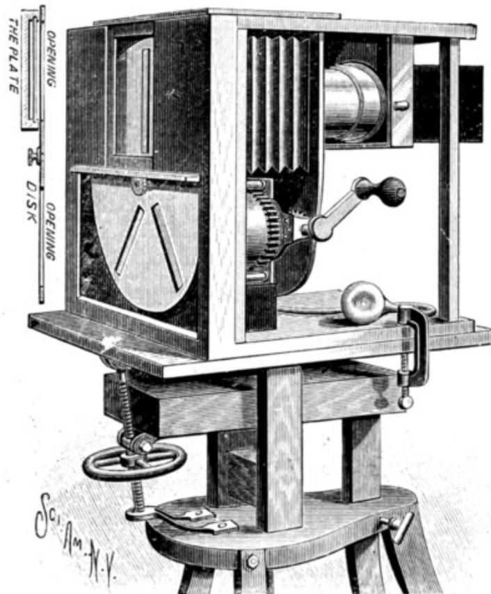
FIG. 4.—CHRONOPHOTOGRAPHIC APPARATUS PRODUCING UPON ONE PLATE
