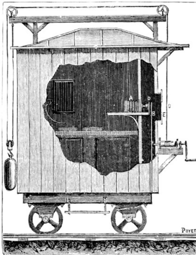
FIG. 7.—INTERIOR ARRANGEMENT OF THE DARK CHAMBER.
