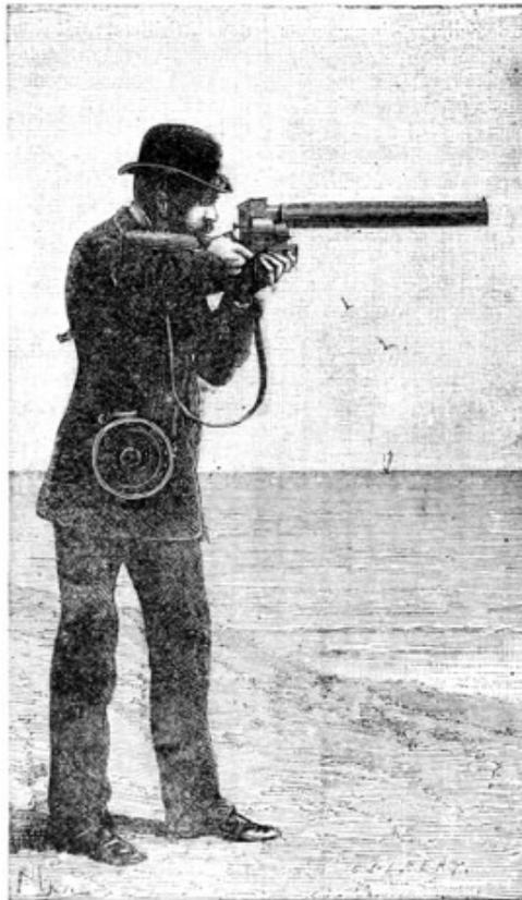
FIG. 17.—MODE OF USING THE PHOTOGRAPHIC GUN.
