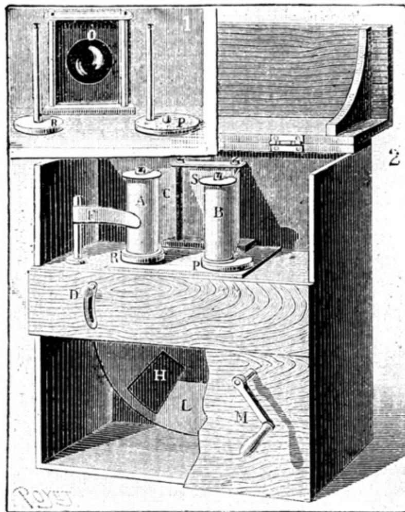
FIG. 1.—AMATEUR'S CHRONOPHOTOGRAPHIC APPARATUS.
