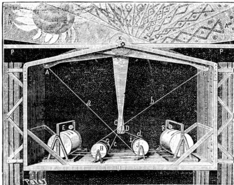
FIG. 2.—APPARATUS FOR MANEUVERING THE FAN.
