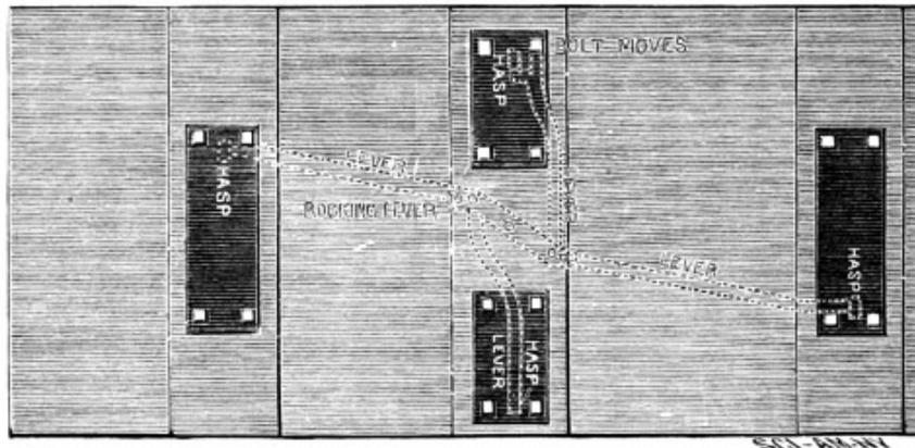
FIG. 3.—BOTTOM OF BOARD, SHOWING PLATES.
