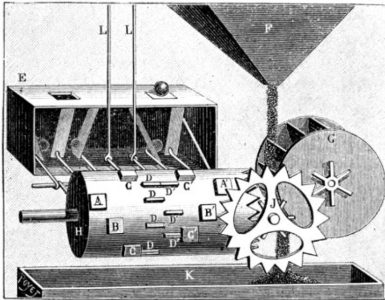
FIG. 2.—INTERNAL MECHANISM OF THE AUTOMATON.
