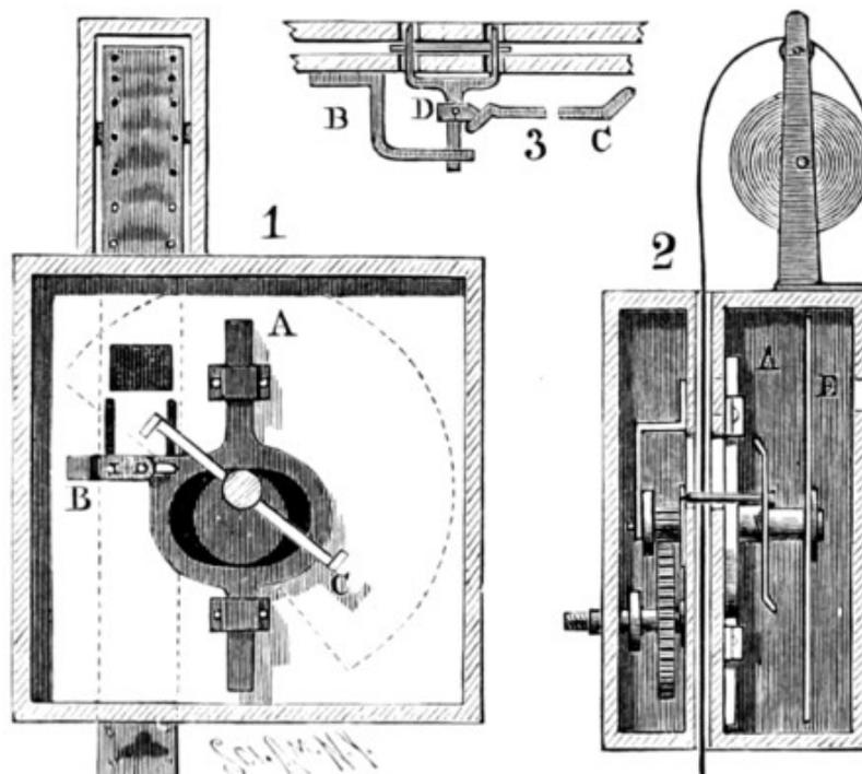
FIGS. 1, 2, AND 3.—FILM-MOVING MECHANISM.
