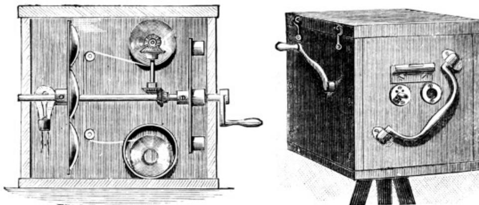
FIGS. 5 AND 6.—THE JENKINS "KINETOSCOPE" CAMERA.
